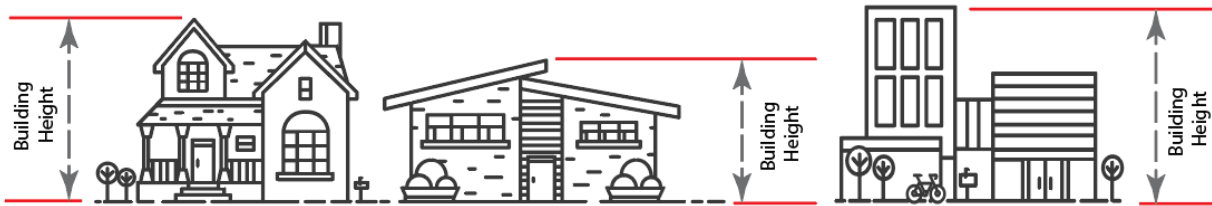
Figure 1105-K: Example of building height measurement.
