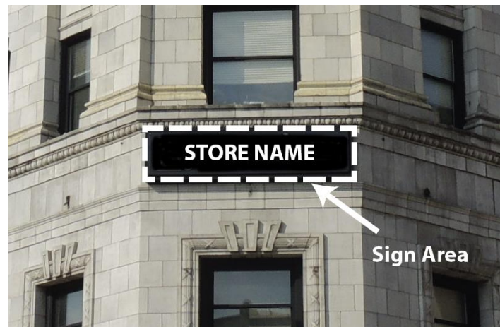
Figure 1113-E: Illustration of computing the sign area for wall signs with a background panel or cabinet.
