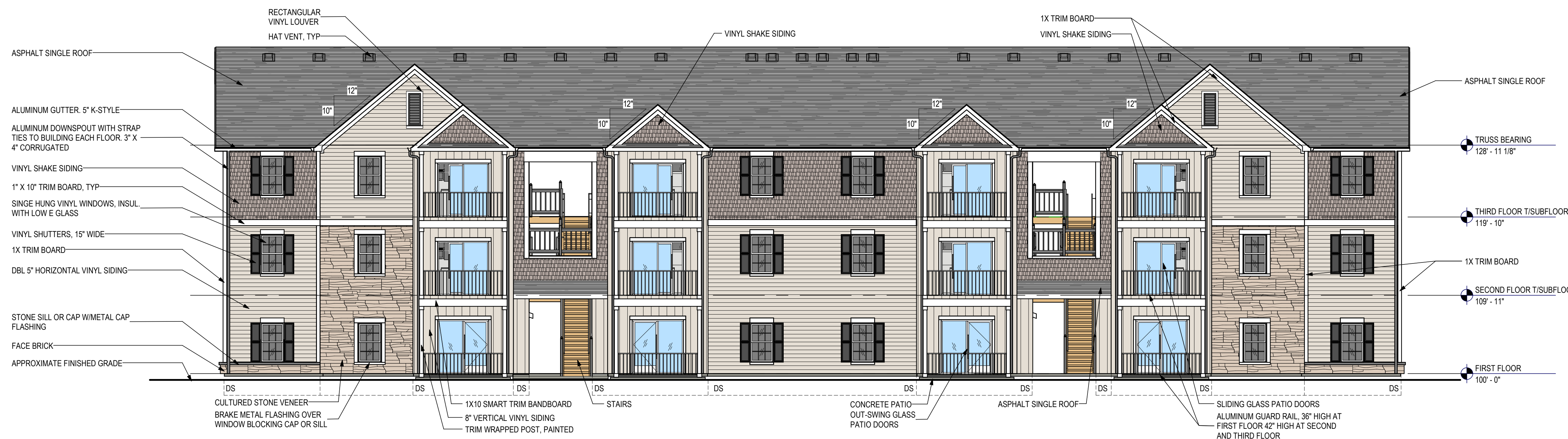
4 south elevation E-1 1/8" = 1'-0"
