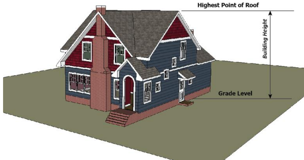
Figure 1105-J: Example of building height measurement.
