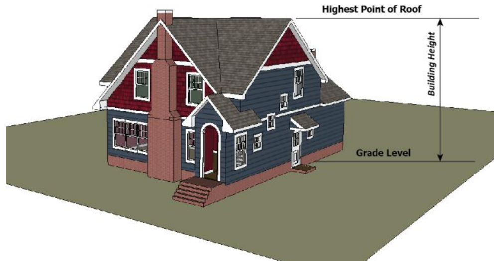
Figure 1105-J: Example of building height measurement.
