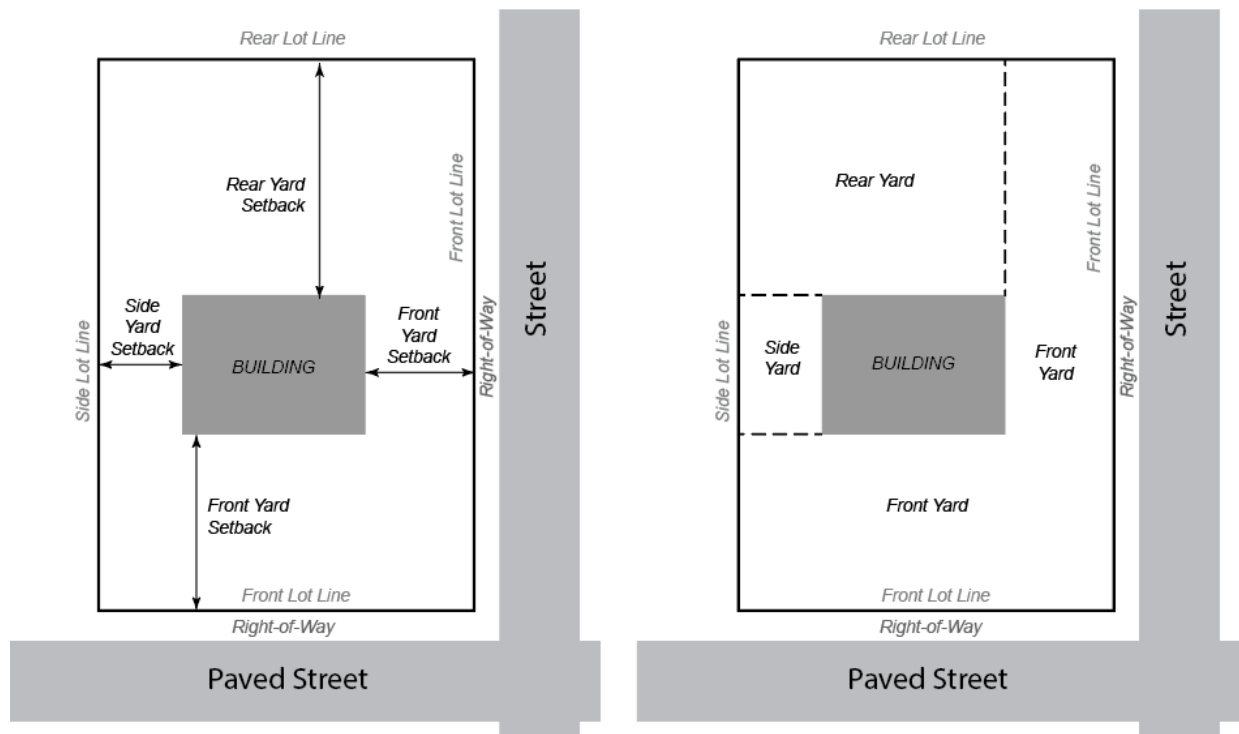
Figure 1105-D: Typical setback and yard locations for a corner lot.
