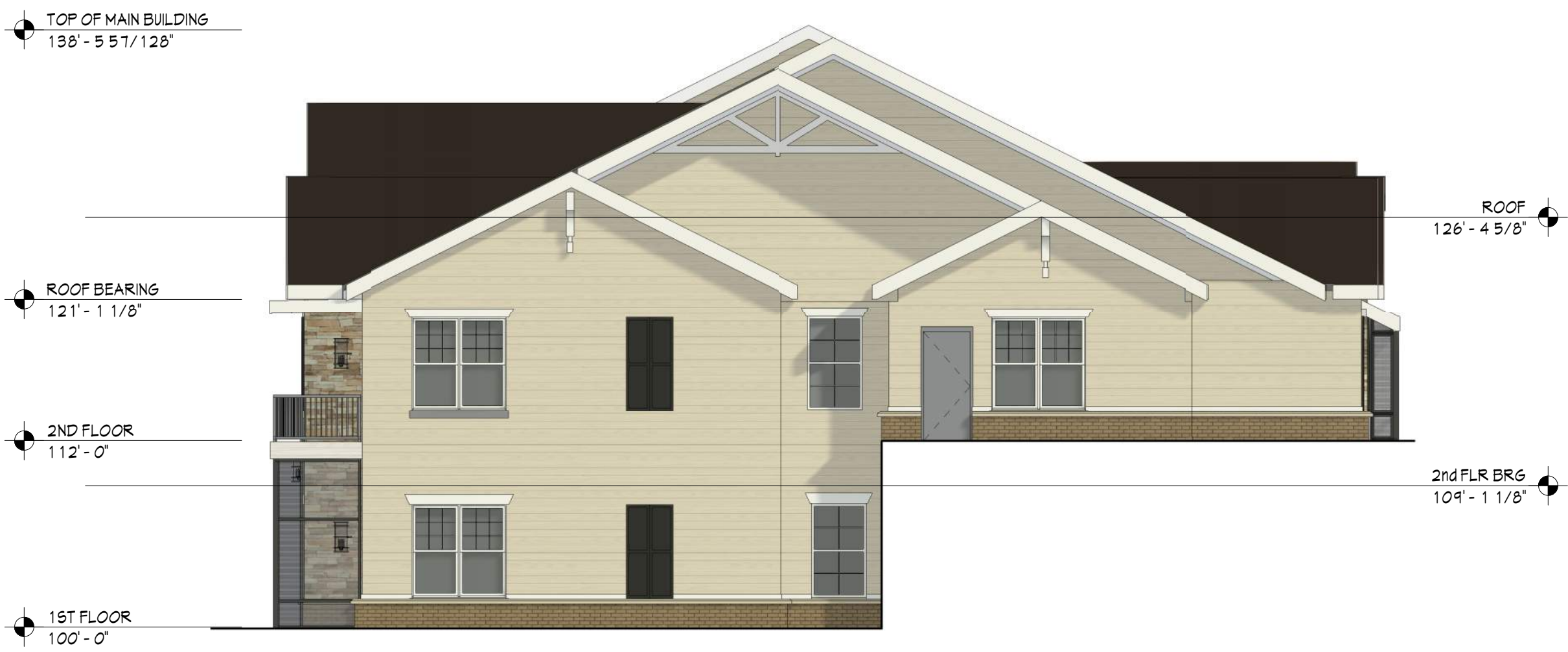
east building elevation
