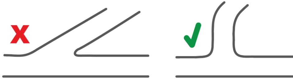
Figure 1114-A: Streets should intersect as nearly as possible at right angles (right image) with the exception of approved roundabouts.
