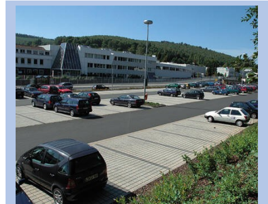
Illustration of porous pavement used in a parking lot to allow stormwater to pass through the pavement.
