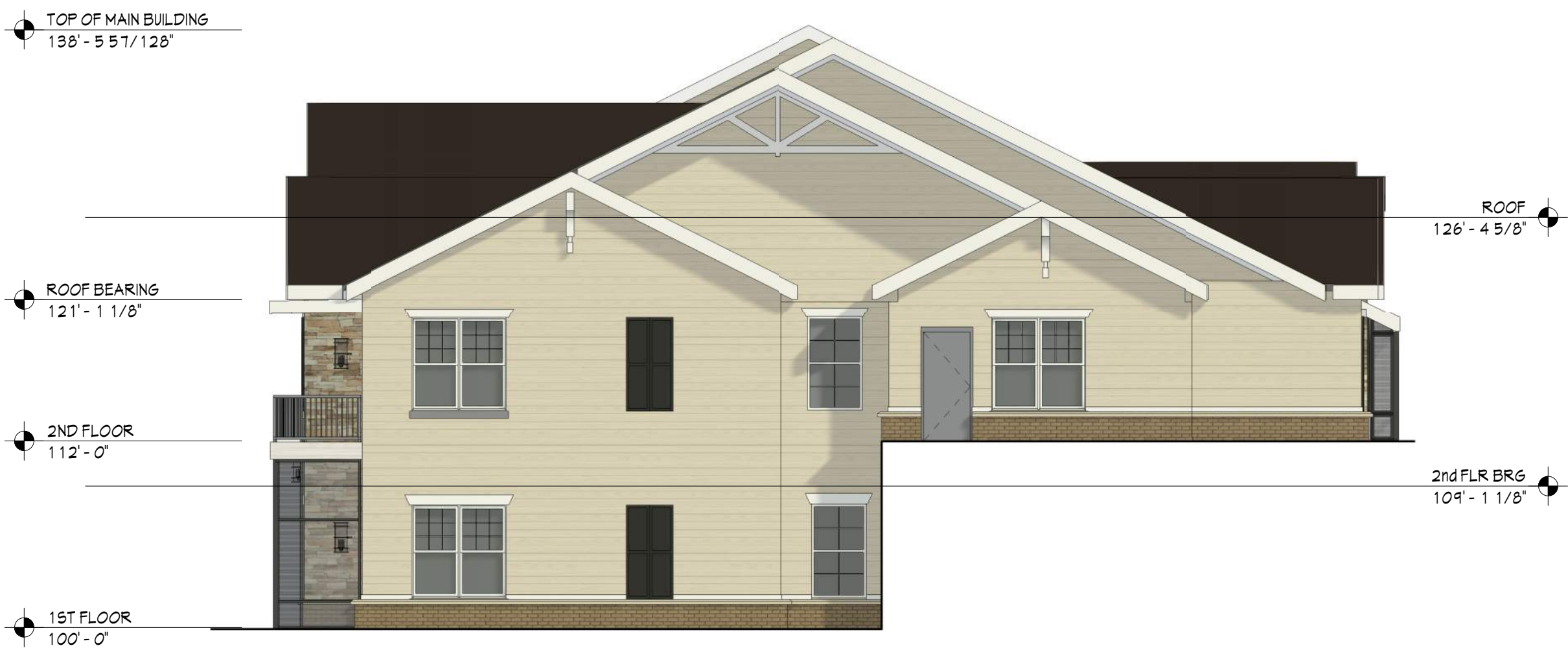
east building elevation 1/8" = 1'-0"
