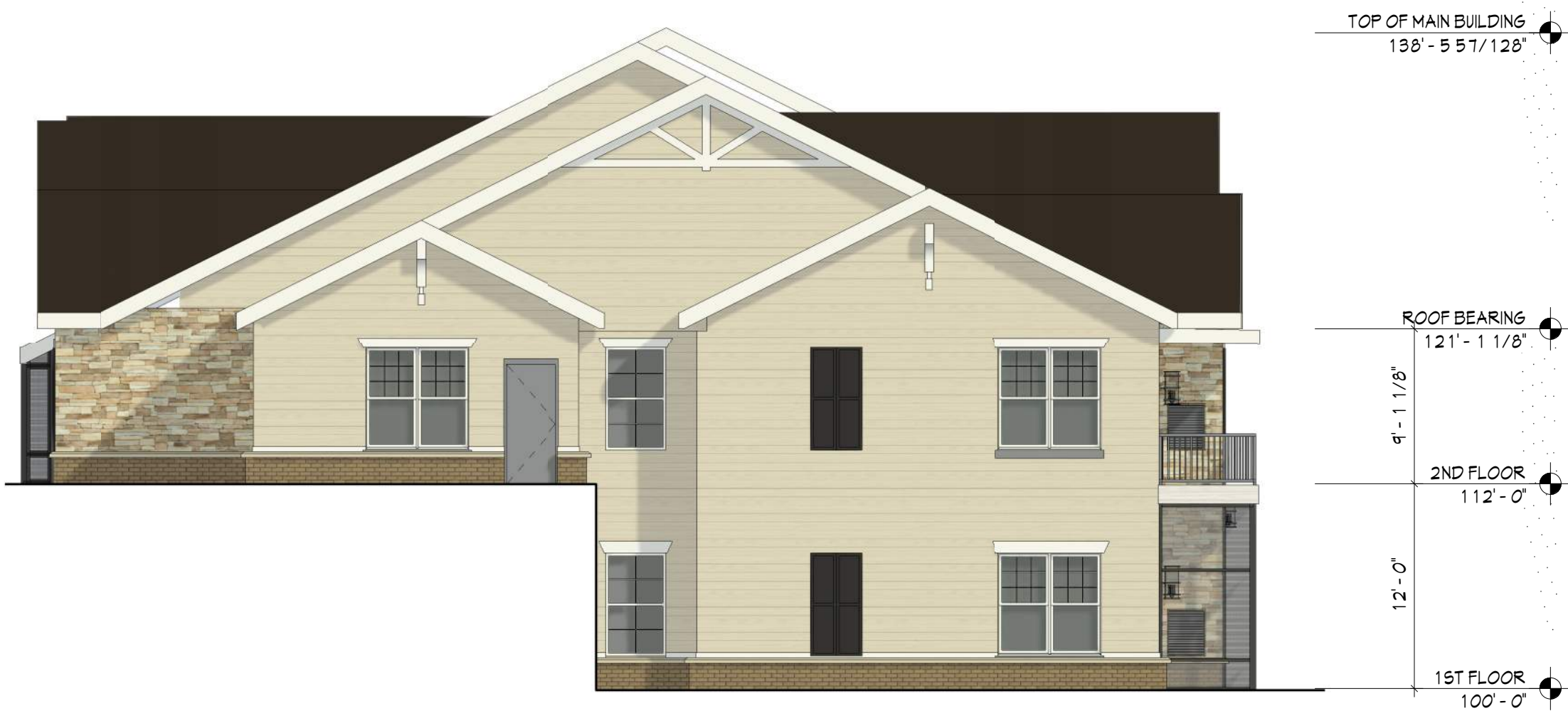
west building elevation 1/8" = 1'-0"
