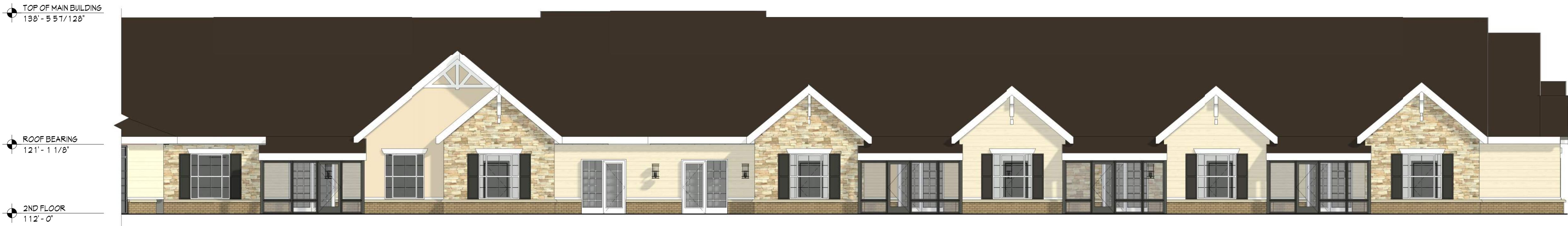
south building elevation - east wing 1/8" = 1'-0"
