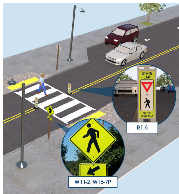
High-visibility crosswalk enhancements Source: FHWA
